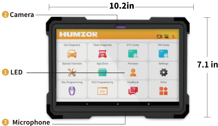
Figure 2-1 NEXZSYS Table Front View
